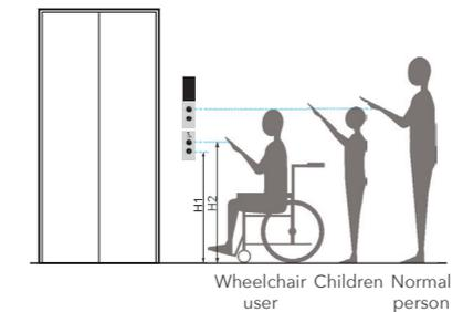
**Note:** Buttons shall be placed at a height that is convenient for visually impaired person, children and wheelchair user. Recommend button height (H1 ~ H2): 900mm ~ 1100mm.
