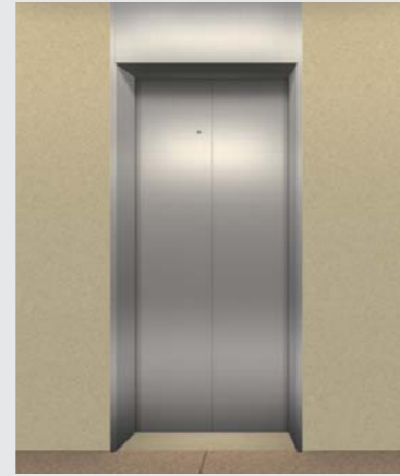
Jamb frame:TL-2X wide type with transom Stainless steel hairline Door panel:Stainless steel hairline Door sill:Extruded hard aluminum
